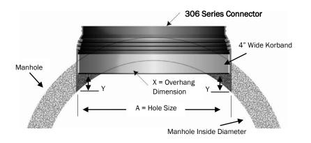
Note Y dimension: Boot must be square in hole (even on both sides).
