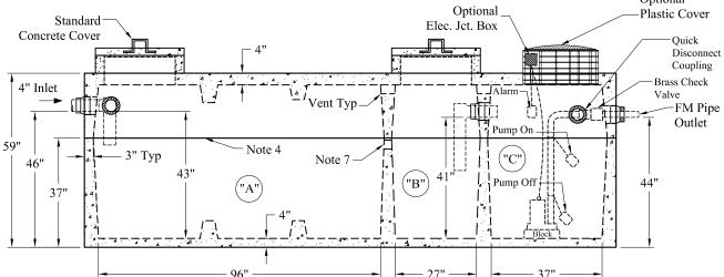
Pumps and Related Accessories are Optional. Junction Box And Electrical Connections Installed By Others
