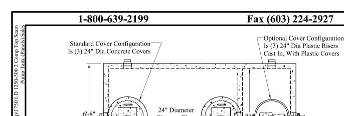
Is (3) 24" Dia Plastic Risers Cast In, With Plastic Covers 6'-8" Cleanout Plugs 3 Places 4" Closed-End **Boot 6 Places** NOTE: A Pipe Bushing Will Be Required On All Boots With Pipes Less Than 4"
