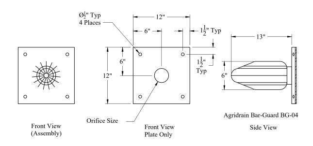
Phoenix Precast Products Trash Racks/Round Structures/Trash Rack for Orifice Less Than 4 Inches (v)
